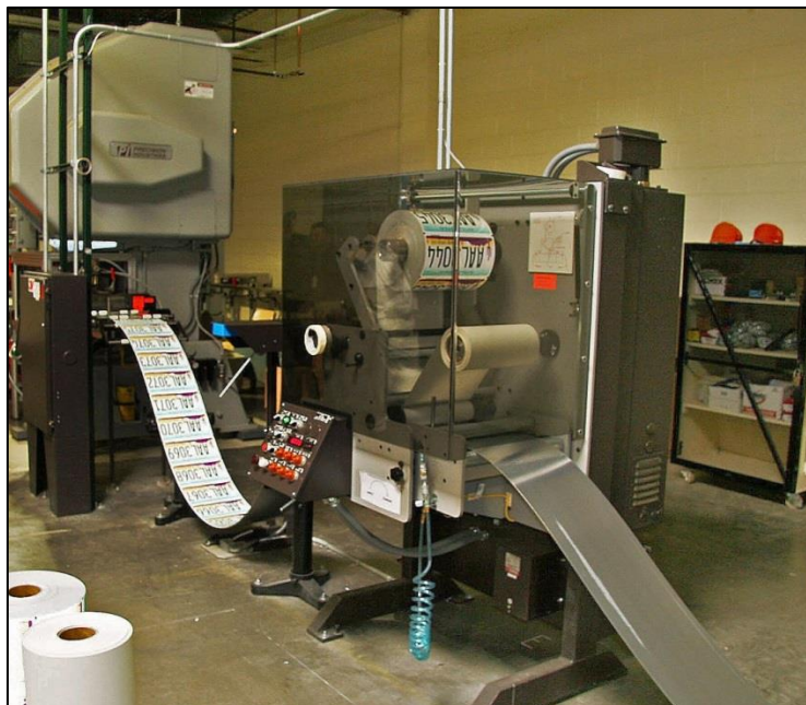
This is how license plates are made today. This blanking line joins the aluminum with the printed vinyl film. At the end of the line is the press that cuts the license plates into their rectangular shape. (Courtesy of ADOT, May 2012)
