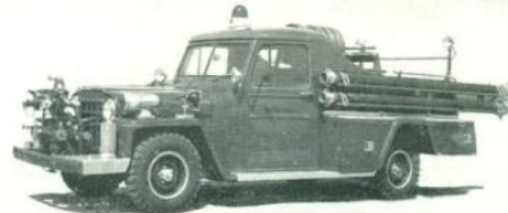
500 GPM triple combination equipment on Model 6-226 Willys 4x4 chassis, 105 HP motor, 118" W.B., Model CF-3 1-stage pump, 150 gal. tank. Body carries 500' 2½" and 330' 1½" D.J. hose. 4 compartments.
