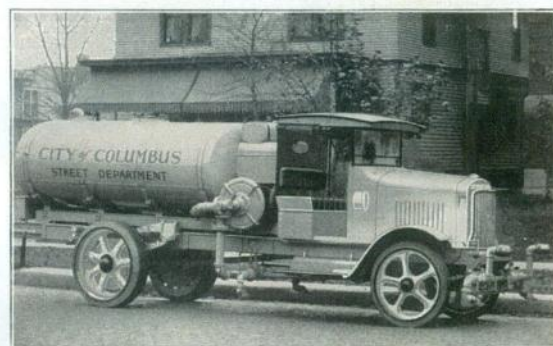
Model 103 International Motor Truck equipped with 1200-gallon Power Flusher and sprinkler attachments.
