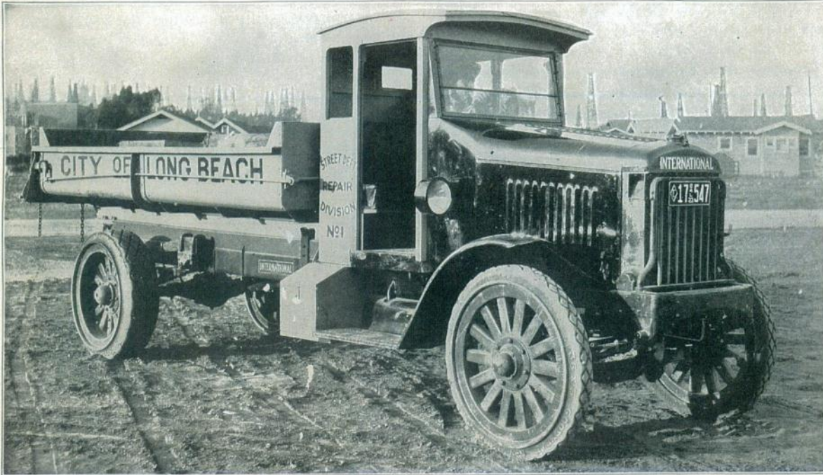
The street department of the city of Long Beach, California, owns this Model 63 International Motor Truck which is being used every day in the repair division of that department.
