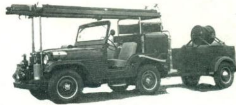
400 GPM triple combination equipment on Model CJ-3B Jeep, 4500 GVW chassis, 70 HP 4-cyl. motor. Model U-40 1-stage centrifugal pump. 200 gal. tank trailer. Body carries 500' 1½" D.J. hose.
