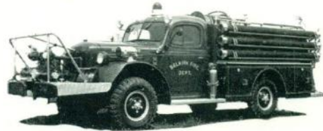
500 GPM triple combination on Dodge Model W-300 4-wheel drive Power Wagon. 126" wheelbase. 125 HP motor. CF-3 500 GPM 1-stage centrifugal pump. 200 gal. tank. Body carries 500' 2½" and 1000' 1½" fire hose. 5 compartments.
