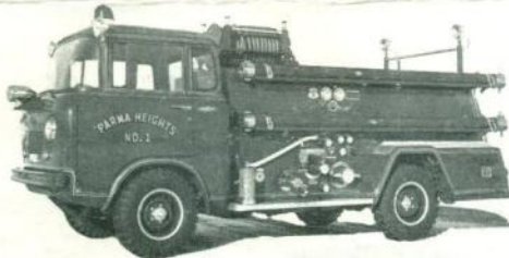
500 GPM triple combination equipment on Willys FC-170 chassis, 105 HP motor, 104" W.B., Model CA-1A 1-stage midship mounted centrifugal pump, 200 gal. tank. Also available with CF-3 1-stage front mounted pump. Body carries 600' 2½" and 300' 1½" D.J. hose. 4 compartments.
