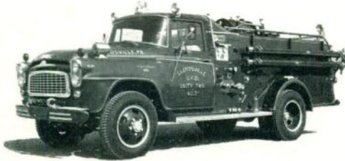
300 GPM triple combination on International B-142 4x4-14,000 GVW chassis. BD-264—153 HP motor. 141" W.B., CP-3 2-stage power takeoff centrifugal pump, 300 gal. tank. Body carries 1000' 2½" D.J. hose. 4 compartments.
