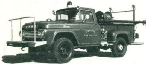
250 GPM triple combination on Ford F250, 7400 GVW, 4x4 chassis. Model 292—186 HP motor. 118" W.B., CP-2 1-stage power take off centrifugal pump. 200 gal. tank. Ford pick-up body, carries 400' 2½" D.J.
